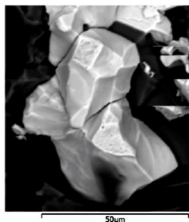
Figure 5. Backscatter scanning electron microscope image of monazite-(Ce) from the Penn/MD Materials quarry. Magnification is approximately 2100 X.
