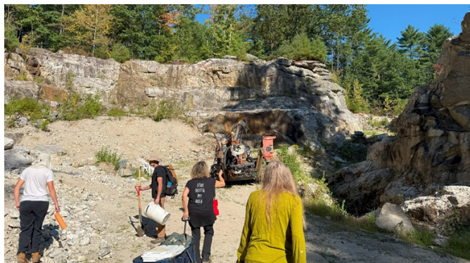
Figure 2. View of the access road at Havey running through the mined out area of the quarry with the spoils to the left. Note the mobile drill used to drill shot holes. Bill Stephens, PG photo.
